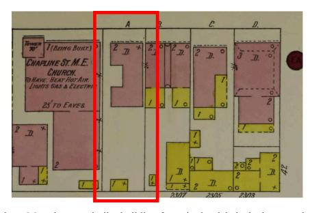
The 1921 Sanborn Map shows a similar building footprint but labels the house as being three stories in height, with a frame front and back porch. Brick evidence supports the addition of the third story on the front portion of the house, while the rear remained two stories.
